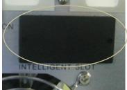
**Step 3:** The cover of AS400 should attach close to the rear panel. Using screwdriver, secure the AS400 to the UPS chassis with 2 screws.
