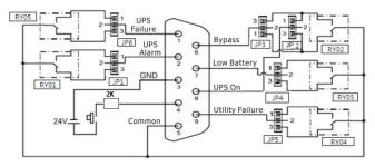
Fig 1 Pin definition and internal logical connection
