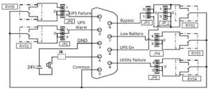
Fig. 3 Connection for ACTIVE OPEN
