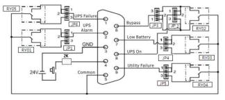
Fig 2 Connection for ACTIVE CLOSE
