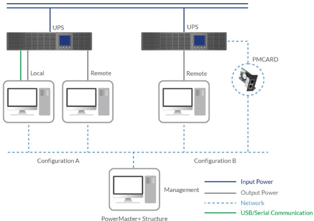
A UPS with a remote management card has the ability to communicate with multiple computers which have Remote installed and are on the same network and relay the UPS status to each Remote. In the event of a power failure, each Remote will request the hosted computer to shut down following notifications from the UPS. Refer to Configuration B of the Power Master+ structure illustration.
